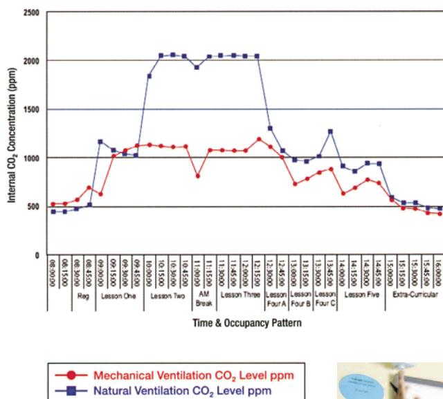
As illustrated on the left, the mechanical ventilation system (**Classvent**) holds the CO<sub>2</sub> levels below the stipulated 1500 parts per million guideline. Data taken from the naturally ventilated room was taken with the windows open and CO<sub>2</sub> levels would rise even further should the windows be closed in the winter months.
